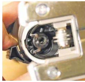
▲ You have to operate the lever to align the collar and fit the blade
